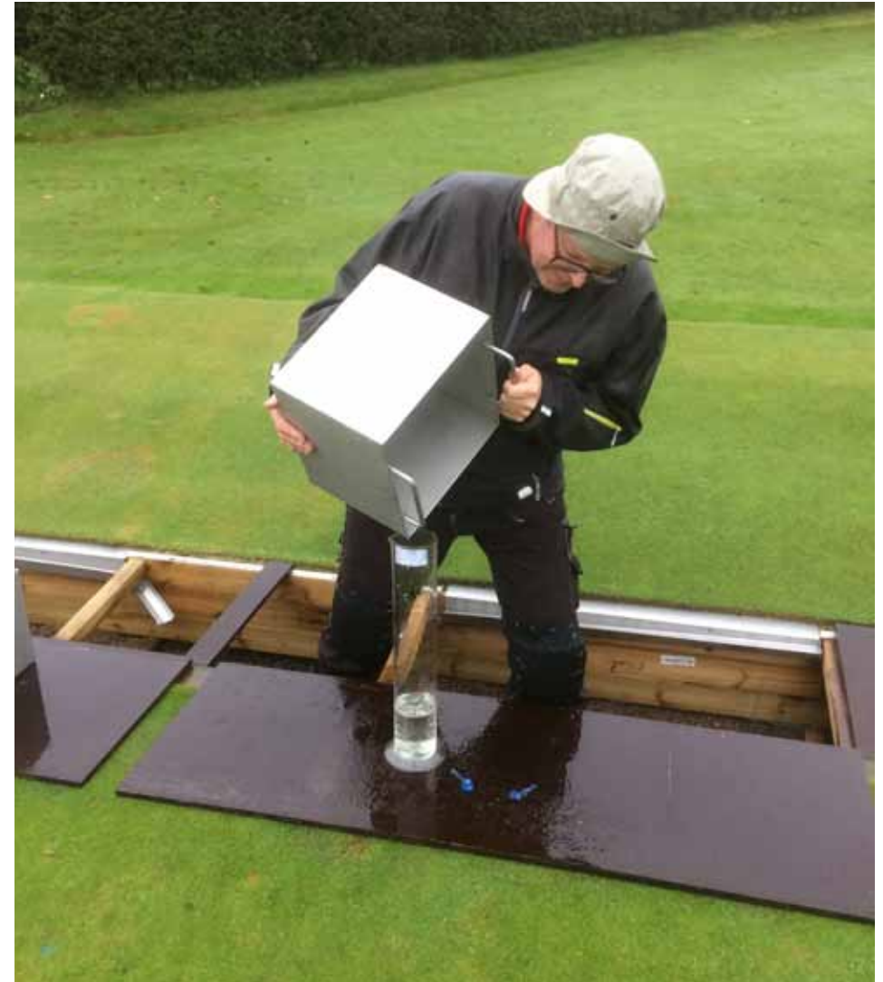
Collection of surface runoff on 20 October 2017, two days after fungicide application. Photo: Trygve S. Aamlid.
