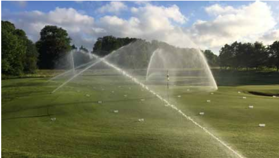
Conducting an irrigation uniformity field test Denmark in June 2017. Photo: C Gómez
